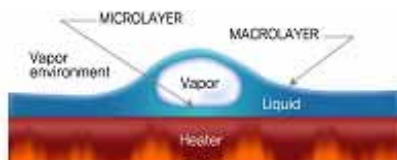
Figure 1. illustration of liquid sublayer structure [7]
