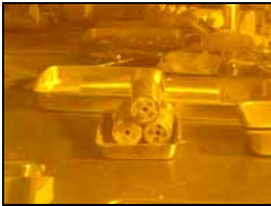
Figure 3. Cut and dismantled thermal media with outer pipe.
