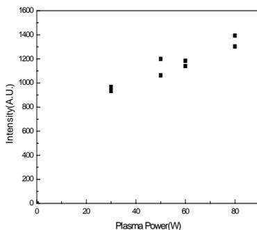
Fig. 4. Variation of Oxygen Intensity as a function of Power in  $O_2 / N_2$  Plasma
