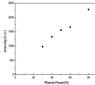
Fig. 5. Variation of Oxygen Intensity as a function of Power in  $O_2 / He$  Plasma
