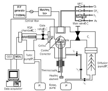
Figure 1. Schematic of plasma oxidation apparatus
