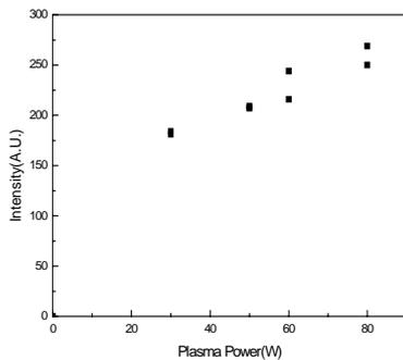
Fig. 3. Variation of Oxygen Intensity as a function of Power in  $O_2 / Ar$  Plasma
