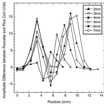
Fig. 2 Distribution profiles of the signal amplitude difference between pancake coil and plus coil at a frequency of 300kHz along the EDM notch length.
