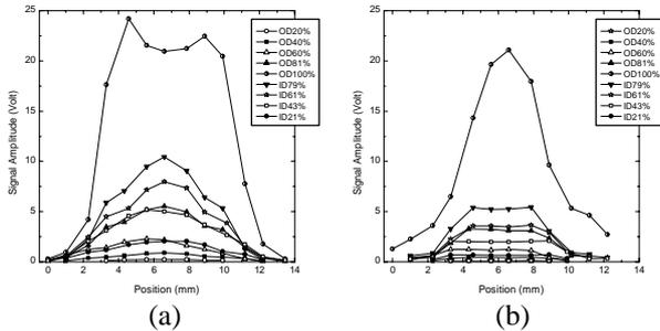
Fig. 1 Distribution profiles of the signal amplitude by (a) pancake coil and by (b) plus coil at a frequency of 300kHz along the EDM notch length of 7mm.
