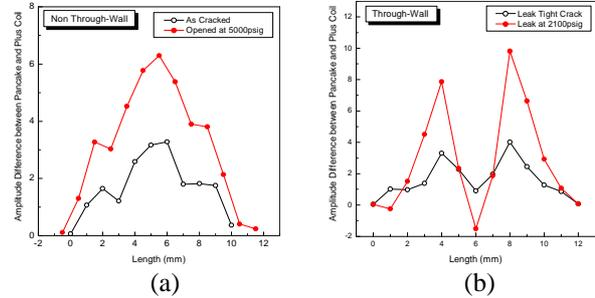
Fig. 3 Verification of the M-shape criterion using the axial fatigue cracks with (a) non-through-wall depth and (b) through-wall depth.
