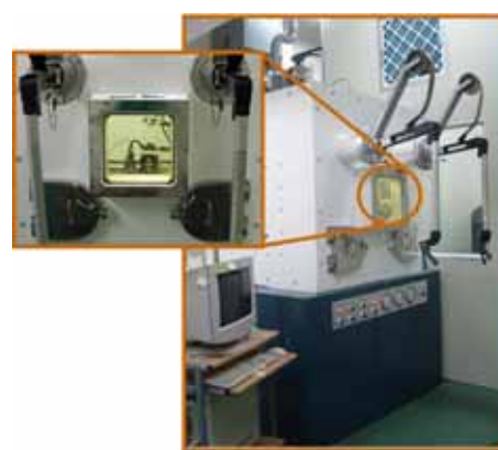
Figure 1. The lead shielded laser ablation system
