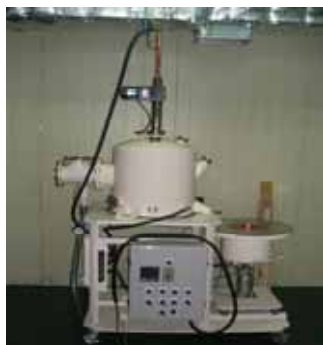
Figure 1. Electric arc melting apparatus.
