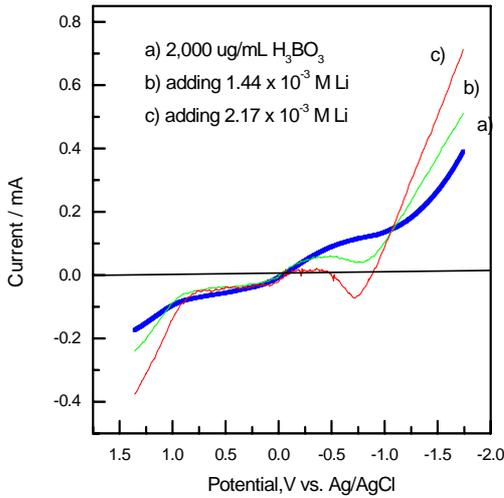
Fig. 2 Linear sweep voltammograms at a Pt electrode in various boric acid solutions
