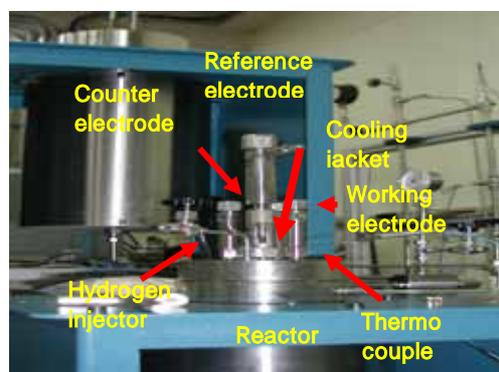
Fig. 1. Equipment of electrochemical autoclave system
