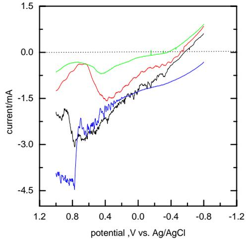
Fig. 4 . Linear sweep voltammograms at a Pt electrode in various dissolved hydrogen concentration in 1200 ppm  $H_3BO_3$  3.0 ppm Li at high temperature, green; 0.09  $H_2$  cc/kg at 288 °C, red; 37.8  $H_2$  cc/kg at 286 °C, black; 59.7  $H_2$  cc/kg at 283 °C, blue; 74.4 $H_2$  cc/kg at 283 °C,
