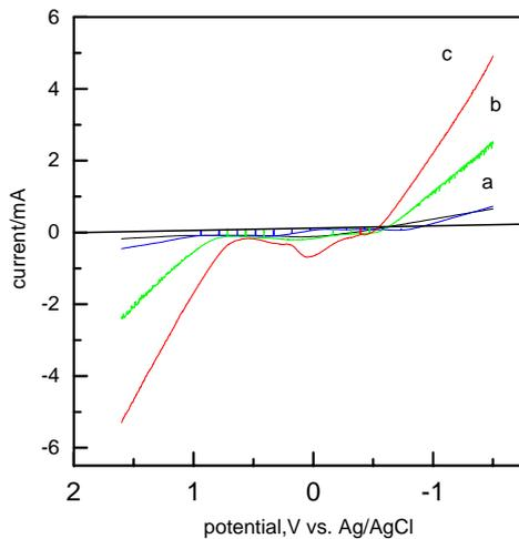
Fig. 3 Linear sweep voltammograms at a Pt electrode in various temperature in  $7.24 \times 10^{-4}$  M  $H_3BO_3$  a);46.6, b);155.9, c)256.7+(o)C respectively
