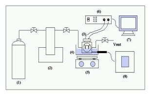
Figure 1. Experimental apparatus ; (1)  $CO_2$  cylinder (2) Syringe pump (3) Reaction cell (4) Water bath (5) Magnetic stirrer (6) RQCM (7) Monitor (8) Temperature controller
