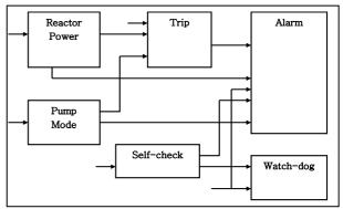
Figure 1. Overall Scheme of Safety Shutdown System implemented by MDD method
