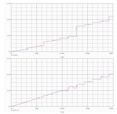
Figure 6. Cadence Spectra simulated result of D-A converting circuit with (a) analog circuit, (b) digital circuit.
