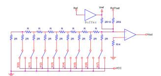
Figure 1. The basic circuit of N-channel ladder network in the general digital to analog converter.
