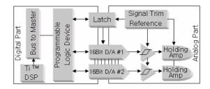
Figure 2. The functional block diagram in the digital to analog converting device.
