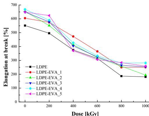
Figure 3. Elongation at break of LDPE/EVA blends as a function of irradiation dose.
