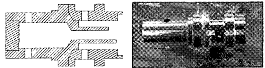
Fig. 1 Double swirl injector for gas generator (Mixed Type, R.N=0.0(#5), 0.5(#6), 1.0(#7))
