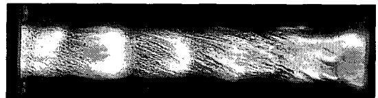
Fig. 1 Photograph of PMMA (swirl intensity = 9.4, after 7 sec burning)
