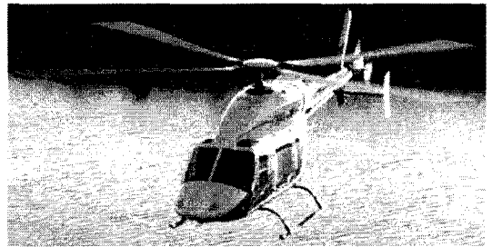
Fig. 1 Sample helicopter figure with skid landing gear (SB427 by Bell Helicopter Co.).
