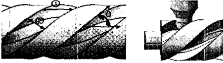
(a) Determination of helix angle (b) Adaptation of tool Fig. 7 Schematic design of formed tool
