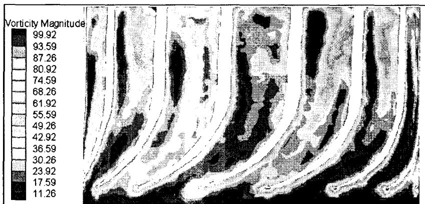
Fig. 3-27 Eddy distribution at vertical section of radius R=3.0\text{m} in the runner channel at condition of H=107\text{m} , a_0=16\text{mm}
