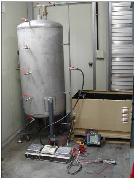
[Figure 5] Power measurement with hotplate [Figure 6] Measuring power generated by gas engine generator
