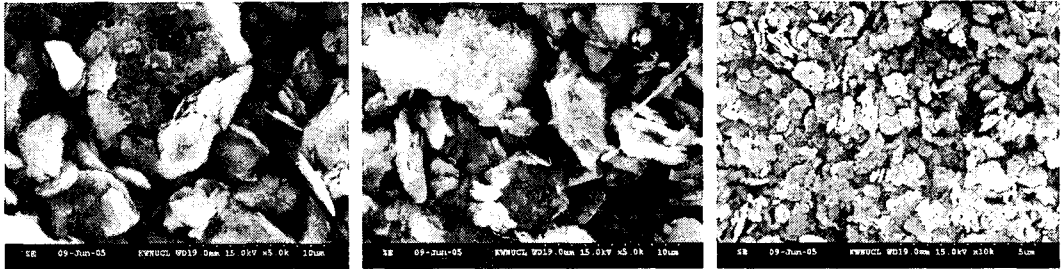
Photo 1. SEM photo of Cotalc-70. Photo 2. SEM photo of Cotalc-90. Photo 3. SEM photo of No.1 Clay.
