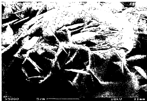
Figure 3. SEM image of katoite (hexagonal in shape) formed from synthetic brownmillerite upon hydration.
