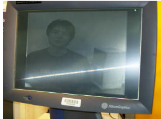
Fig. 8 8-view image for the test image of 'Man' on the commercial 3D display monitor of SiliconGraphics
