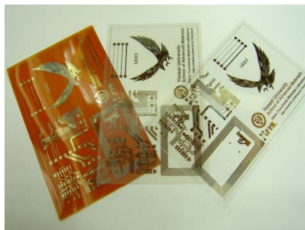
Figure 6 Various patterns ink-jet printed using Ag nano-particle on polymeric substrates.
