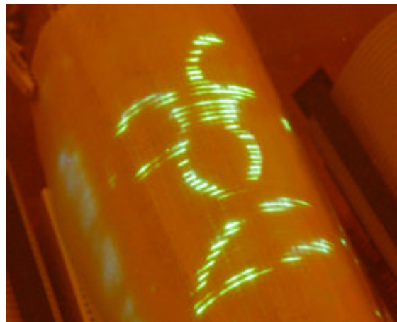
Figure 6: The preliminary image of a cartoon character on the PET flexible substrates under an intentional bent.
