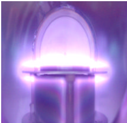
Figure 2. RF-plasma treatment phenomenon using Ar gas.
