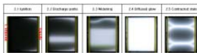
Figure 2. Visible image of the long gap discharge progress with increasing driving voltage
