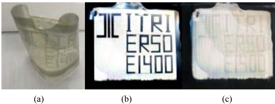
Figure 2 A 4.1 inch film-like LCD operated in the TN mode. (a) photograph (b) on state and (c) off state.
