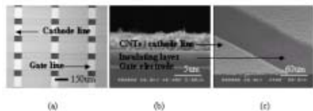
Figure 3. An optical microscope image and SEM images of triode structure.
