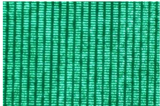
Figure 5 The pixel emission pattern of the test manufactured FED panel.
