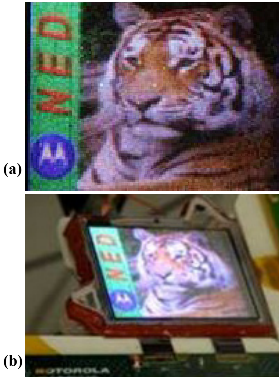
Figure 3. A sealed nanotube-based field emission display showing color images of a tiger, top-down (a) and at an angle (b). Images were produced with a 45 V column swing, 90 V total on the gate electrode, 4400 V on the anode, using a 1.1 mm anode-to-cathode gap. The anodes were fabricated by TECO Nanotech Company.
