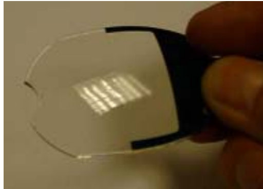
Fig 2: The reduction in light intensity and the desired diffusion of the reflected light are apparent in the half that includes the molded MARAG™ component.
