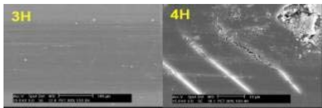
Figure 5: SEM images of OC-LR coating surface on hard coat after pencil hardness testing with 3H and 4H pencil.
