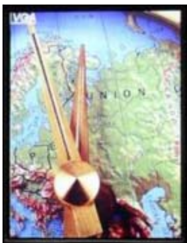
Figure 4. 2” VGA PenTile RGBW display with 400 ppi (Courtesy: Samsung AMLCD Div.)
