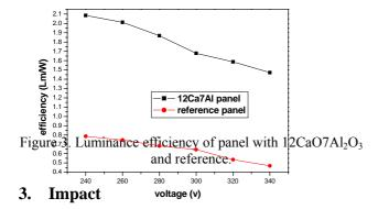
With the use of electride powder at the surface of dielectric layer as electron emission layer, luminance and luminance efficiency of PDP was enhanced about 200-300%. The low work function value of the material is believed to have promoted the electron emission, eventually improving luminance and luminance efficacy. This work demonstrated a possibility of using new class of material as electron emission layer for PDP.
