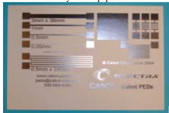
Figure 1. Example of Ink Jettable Silver nanoparticle ink capabilities. This image is an example of Cabot Corporation's Customer Demonstration coupon printed on medium density coated paperboard.
