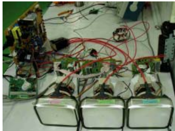
Fig. 6 Photograph of the horizontal deflection board, three projection picture tubes and their driver board.
