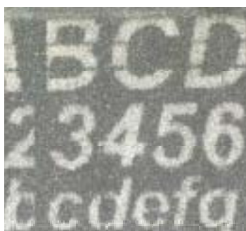
Figure 7. Reflective display fabricated from a 128x128 printed polymer TFT array with gyricon media.
