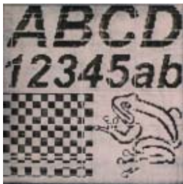
Figure 6. Reflective electrophoretic display made using the printed TFT backplane.
