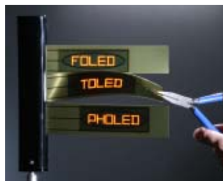
Figure 4. Examples of thin film encapsulated phosphorescent TOLED icons demonstrated at the 2004 SID conference by UDC, Vitex Systems and PARC.
