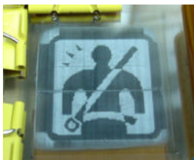
Figure 7: 120 \times 120 array of pixel, 2.4-inch panel image of the toner type PLD device
