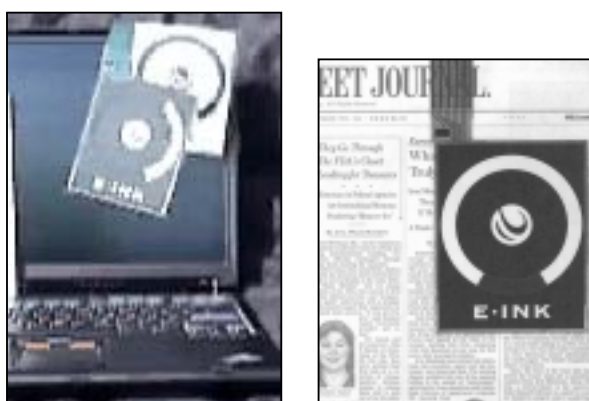
Figure 1a (left). An E Ink flexible segmented display on PET is compared to a newspaper in office light.
