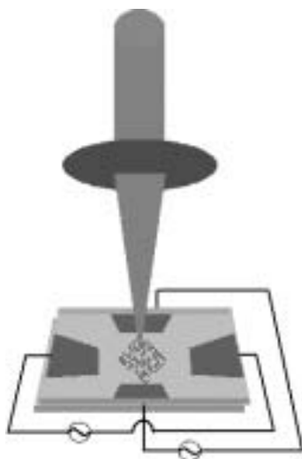
Figure 3. Schematic diagram of the switching experiment with applying electric field and irradiating laser light simultaneously. Cell was maintained at the constant temperature and small limited region in the pattern was irradiated with the focused laser light. For switching the limited region only, both strength of electric field and laser power were controlled.
