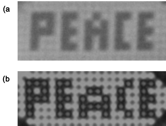
Figure 4. Images under the polarizing optical microscope for two unit domain sizes. The scanning direction of a unit domain had an angle of \pi/4 or -\pi/4 to the horizon and the rubbing of the counter slide was controlled along a scanning direction. The orientations of the polarizers were adjusted for clear images. Contrast and brightness of the images were adjusted for clarity. (a) Unit domain : 1.8\mu\text{m} \times 1.8\mu\text{m} . With dye-added LC. (b) Unit domain : 4\mu\text{m} \times 4\mu\text{m} . With dye-added LC. Cell gap was about 10\mu\text{m} .
