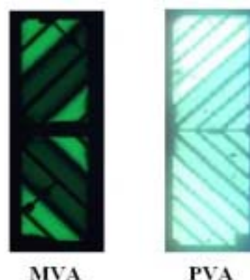
Figure 3. One pixel structure of the MVA & PVA modes with 8-domain.
