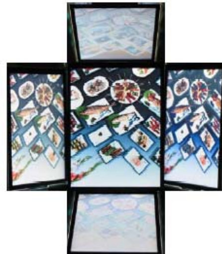
Fig.10 Comparison of display image between IPS and TN mode(WV-film).
