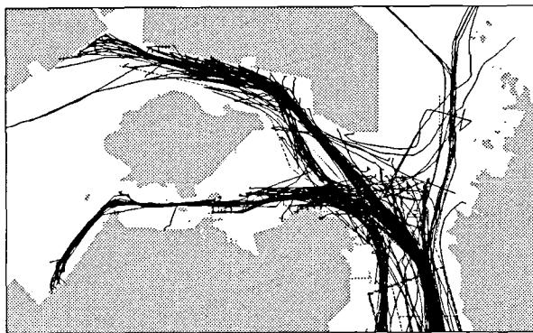
Fig.2 The traffic flow and pattern for incoming vessels in kwangyang harbor
