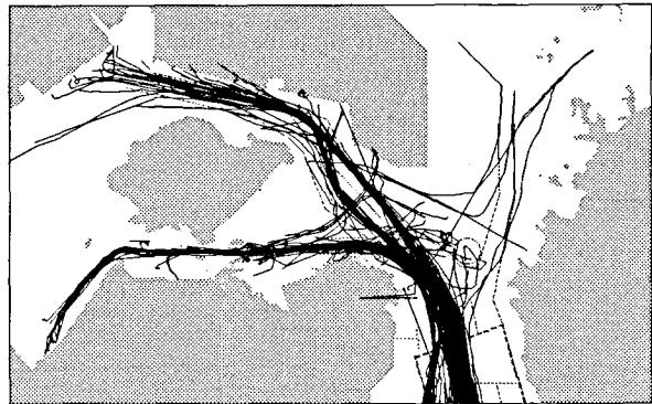
Fig.3 The traffic flow and pattern for outgoing vessels in kwangyang harbor
