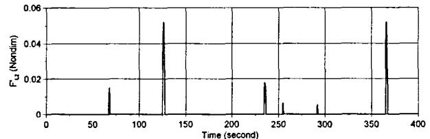
Fig. 6 Nondimensional tension of lashing wire in case of light condition and vertical lashing pattern
