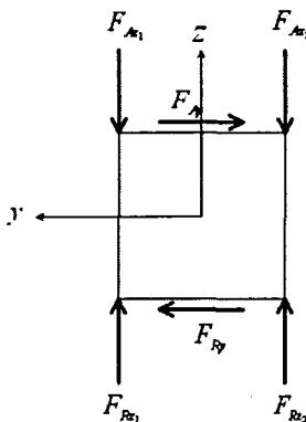
Fig. 2 External surface force acting on a container
