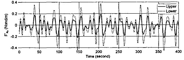
(c) Horizontal reaction force at bottom surface
