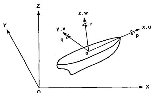
Fig. 1 Definition of coordinate systems and motion variables
