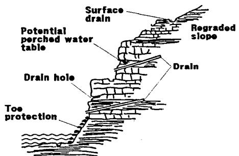
Fig. 6 Cliff draining to reduce water content and pore water pressure
