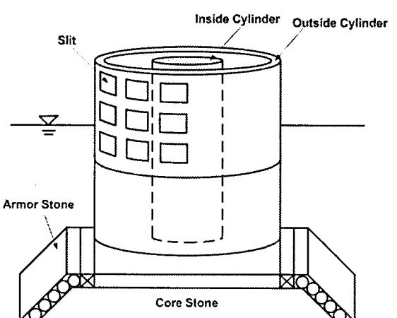
Fig. 14 Aerial view and definition sketch for Cellblock breakwater
