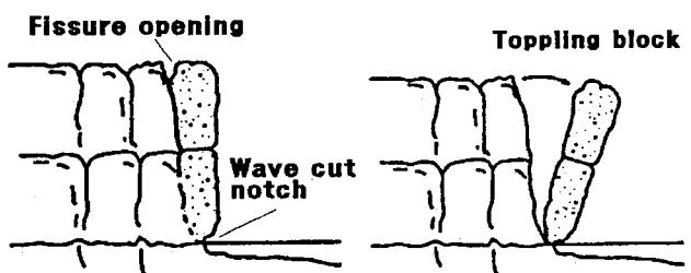
Fig. 3 Failure mechanism of toppling failure
