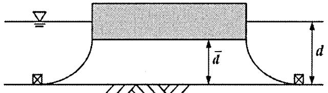
Fig. 13 Definition sketch for floating breakwater
