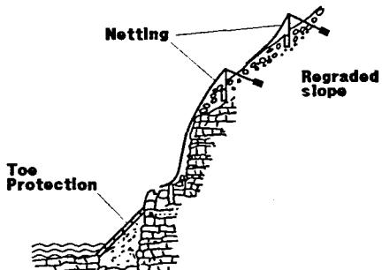
Fig. 7 Netting to reduce impact of falling blocks
