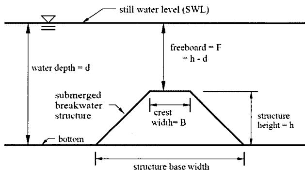
Fig. 12 Definition sketch for artificial reef
