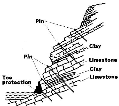
Fig. 5 Rock bolting to clamp rock layers
