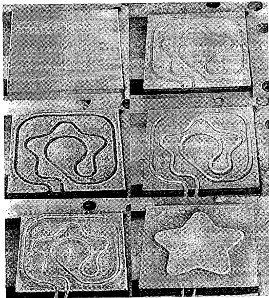
Fig. 11 Process of a conformal cooling manufacturing
