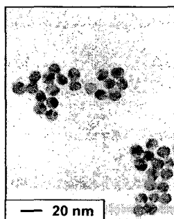
Fig. 4 TEM(Transmission Electron Microscopy) image of Au nanoparticles(size at 13nm)
