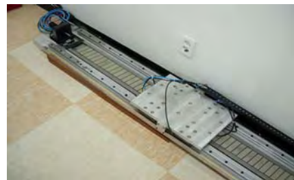
Fig. 10 Product of linear motor system
