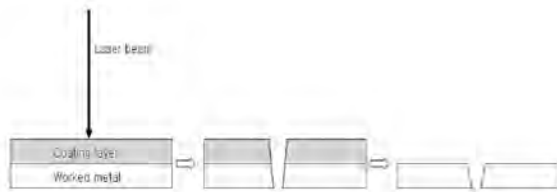
Fig. 4 Process of coating, laser treating and removing coating layer
