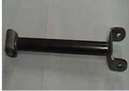
Photo. 2 Top view of trailing Arm
