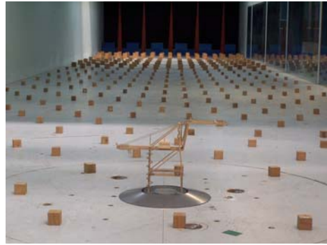
Fig. 3 An articulation type container crane model for wind tunnel test
